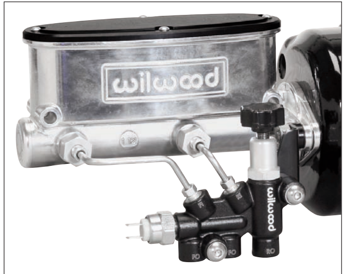
Photo 1. Proportioning Valve Bracket Kit Final Installation
