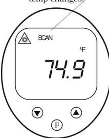
Pull trigger to turn ON. Hold trigger 1 sec., release trigger to HOLD - temp holds.
